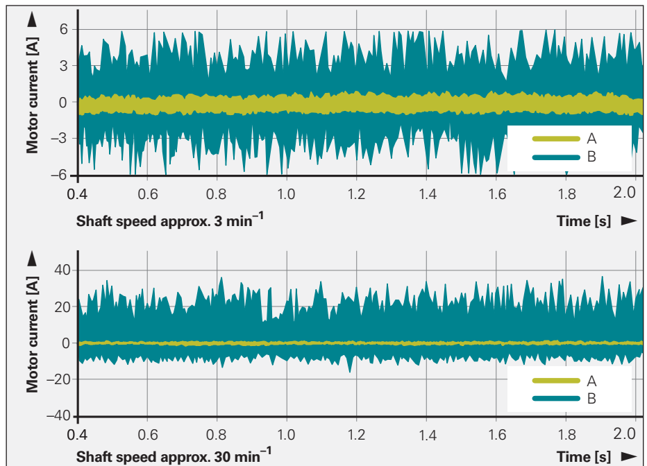
Motor current of a direct drive with position encoder
